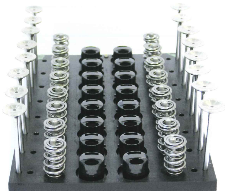
The valves, double valve springs and DLC-coated domed tappets before engine assembly
