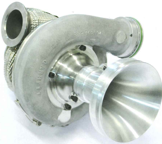
Garrett turbocharger fitted with coned inlet and mandatory 45 mm restrictor
